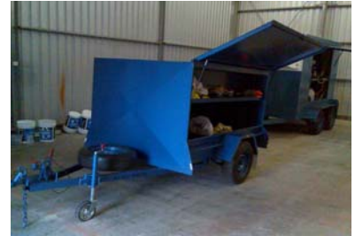
The latest edition to the fleet is this custom built trailer designed to carry 2x205ltr drums of product. The design has been specifically around the quick application of our flooring systems.
